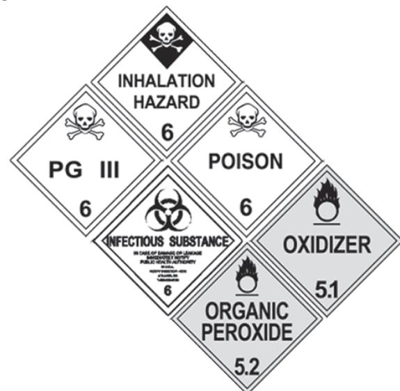
**Figure 9.2** HAZMAT Labels Examples
