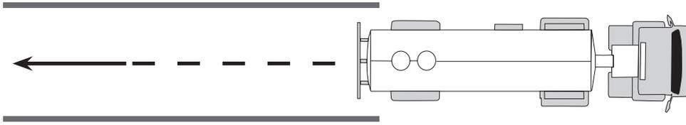
**Figure 12.1: Straight Line Backing**
